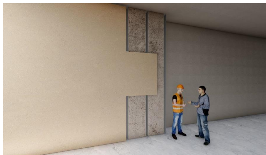
Figure 1 c): Eutectic PCM can be incorporated inside the drywall for use in interior walls which makes it less costly and has high thermal storage as compared to conventional walls.
